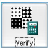
Click the Verify Icon to capture and analyze the image. The image will be analyzed and the actual measured dot areas of the four patches will be displayed. The screen ruling will be displayed as well.
