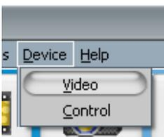
The Device Menu gives direct access to the Video Driver and FLEX<sup>3</sup> sensor. This can be used to diagnose problems or to change the shutter speed and gain for very special applications. Use this function with care. Making measurements with non-factory settings can lead to misinterpretation of the measurement result. A restart of the software always resets the parameters to the factory settings.
